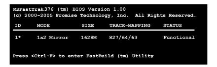
7. Use the FDISK utility and follow the format procedure to install a new hard drive. After you have formatted the arrayed drives, install an operating system (OS).
